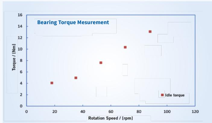
Figure 3: Torque of the Bearing at Different Speeds
