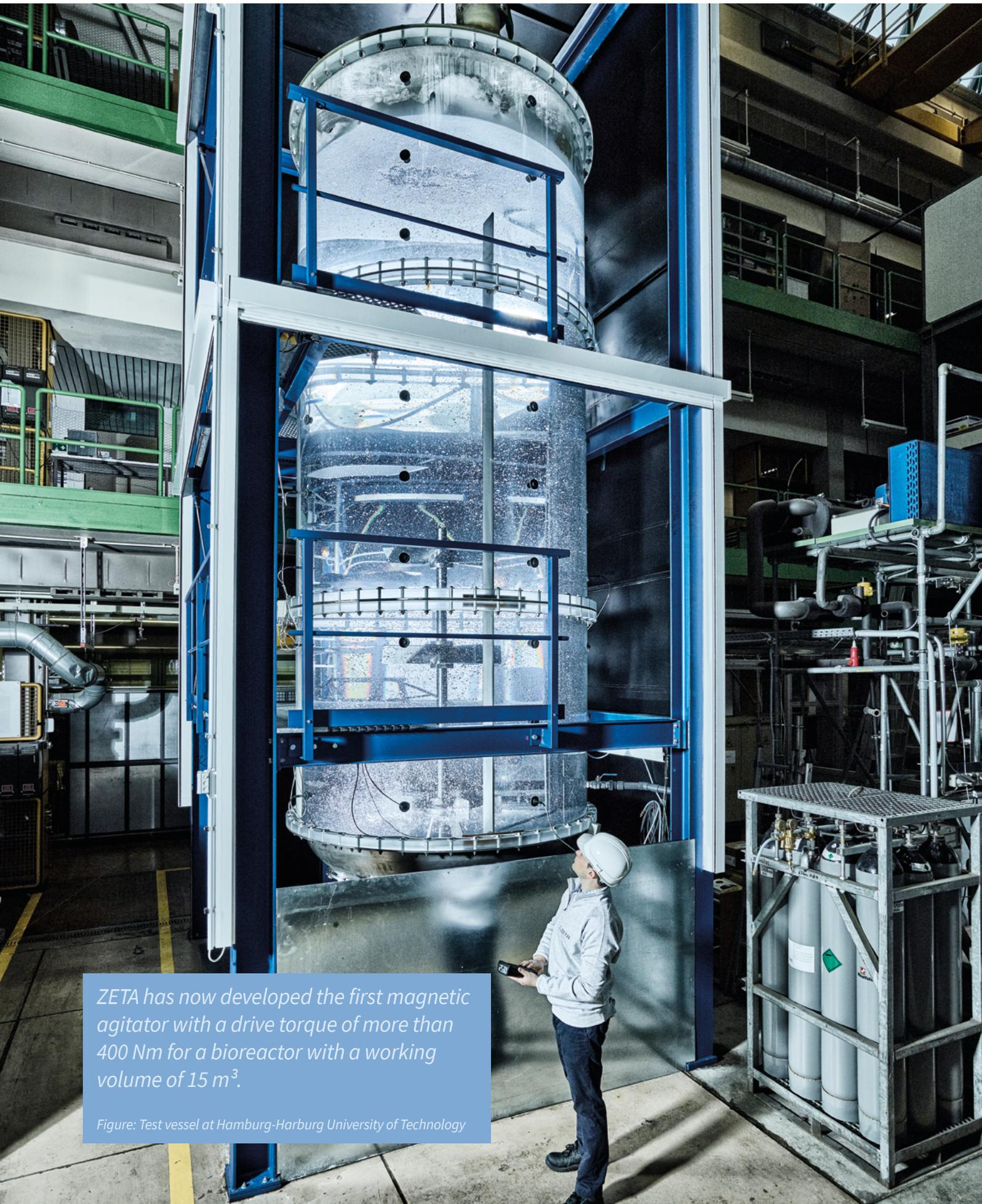
*ZETA has now developed the first magnetic agitator with a drive torque of more than 400 Nm for a bioreactor with a working volume of 15 m<sup>3</sup>.*
