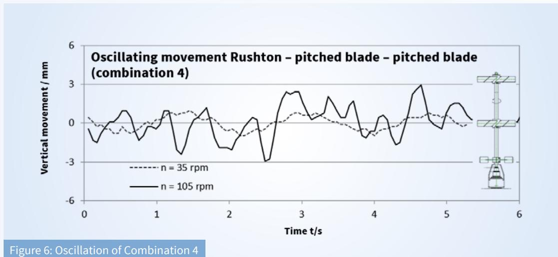
Figure 6: Oscillation of Combination 4
