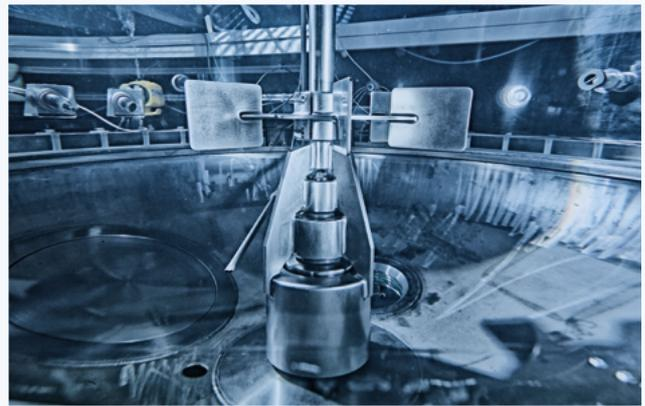
In order to measure the actual power input of each impeller combination into the liquid, it is necessary to know the loss of power generated by the bearing. To do this, the agitator is submerged in water with the water level lying slightly above the agitator shaft. Then the power input of the agitator is measured at different rotational speeds.
