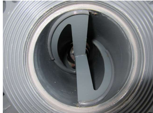
PVC static mixer with steel backing flanges and one side stream injector
